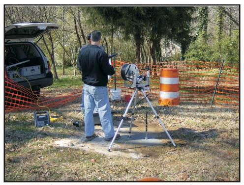
Camera being lowered through cap into well shaft.
