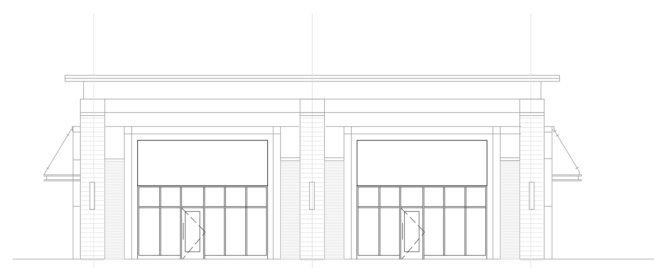
4 SOUTH ELEVATION \frac{1}{8}'' = 1'-0'' SOUTH TRANSPARENCY Total = 23% Total between 3' & 8' = 50%
