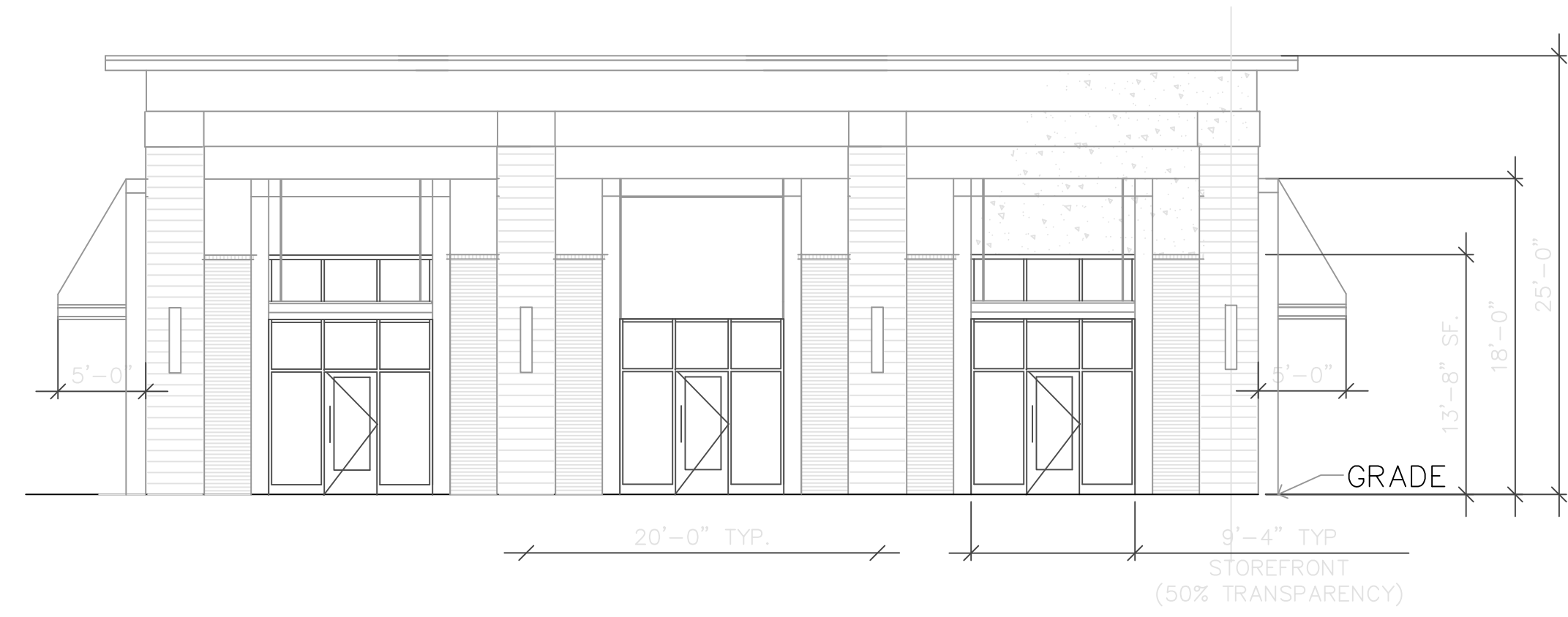
4 SOUTH ELEVATION \frac{1}{8}'' = 1'-0'' SOUTH TRANSPARENCY Total = 23% Total between 3' & 8' = 50%
