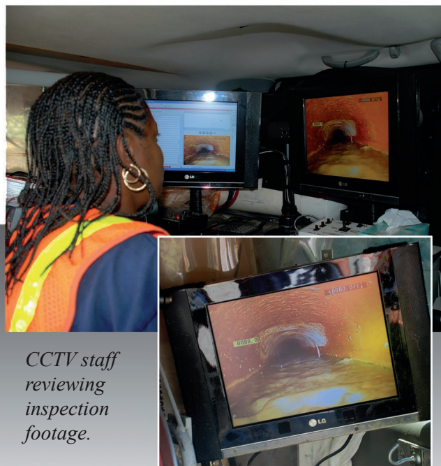
City of Raleigh CCTV crew preparing to inspect a sewer main for damaged or broken lines.
