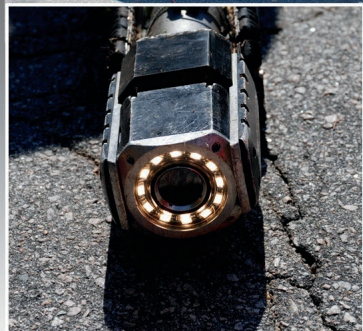
City of Raleigh CCTV crew preparing to inspect a sewer main for damaged or broken lines.
