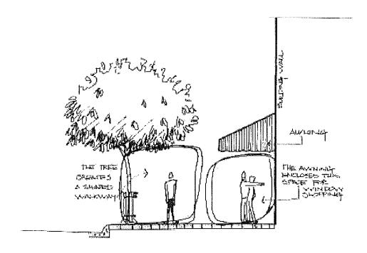
FIGURE 4. TWO-SPACE STRUCTURE USING AWNING AND TREE
