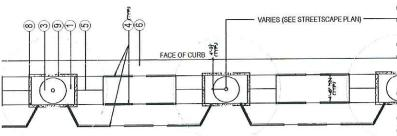
① TREE PIT OPENING 6'-8" x 4'-0" (TYP.) ② 4" PVC DRAIN PIPF IN STONE DRAIN SUMP WRAPP
