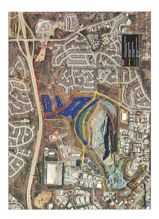
300 Access Road, etc. 40 115' Initial Offset Additional 75' Buffer 300 NOTE: (1) Location of overburden subject to site conditions, engineering and state regulations (2) New location of Westgate Road subject to NCDOT approval Blue Line is Ultimate Quarry Pit Limit RALEIGH DURHAM QUARRY Relocated Westgate Road
