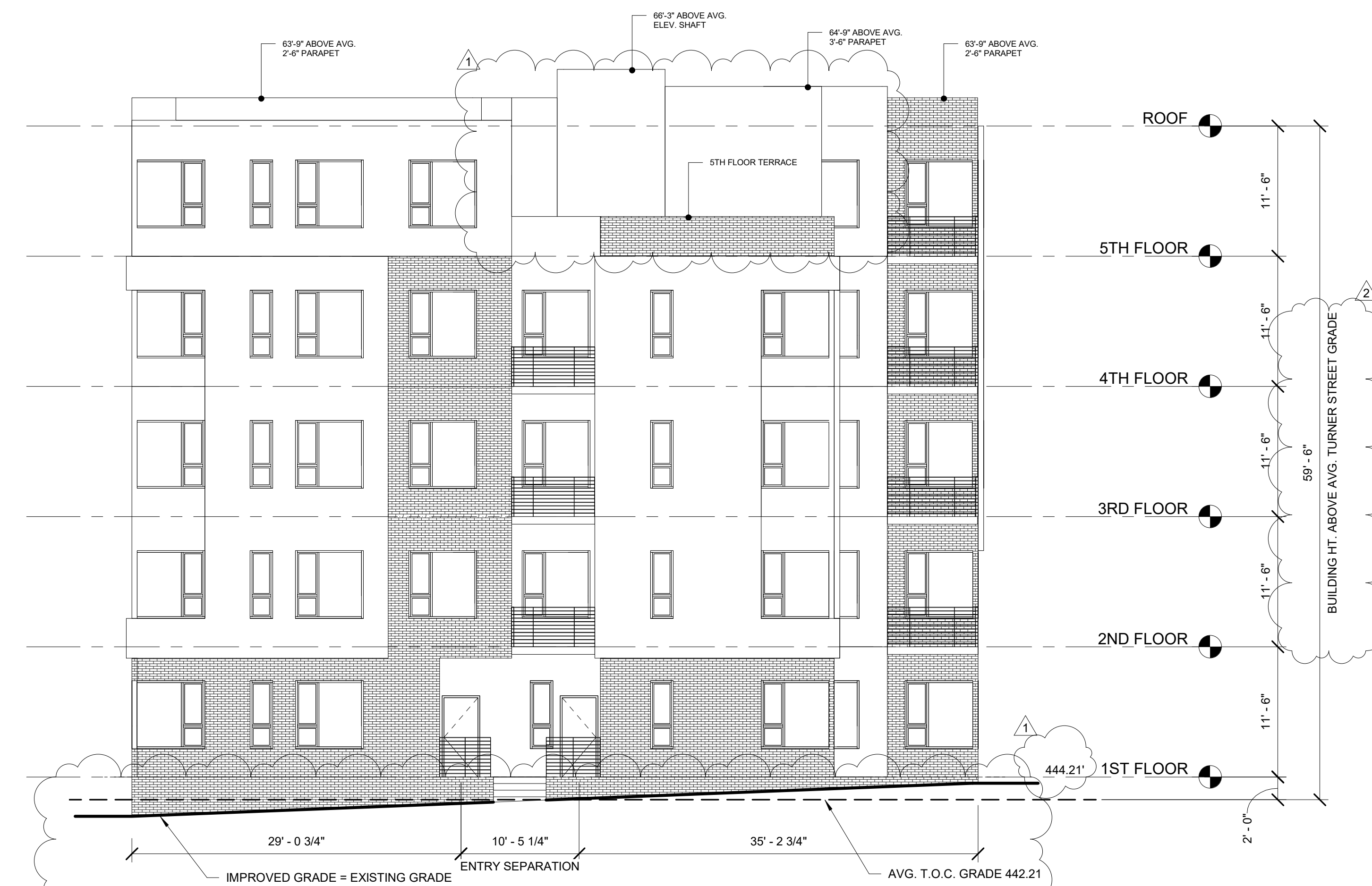
BUILDING (B) EAST ELEVATION 2 TURNER ST. ELEVATION 1/8" = 1'-0"
