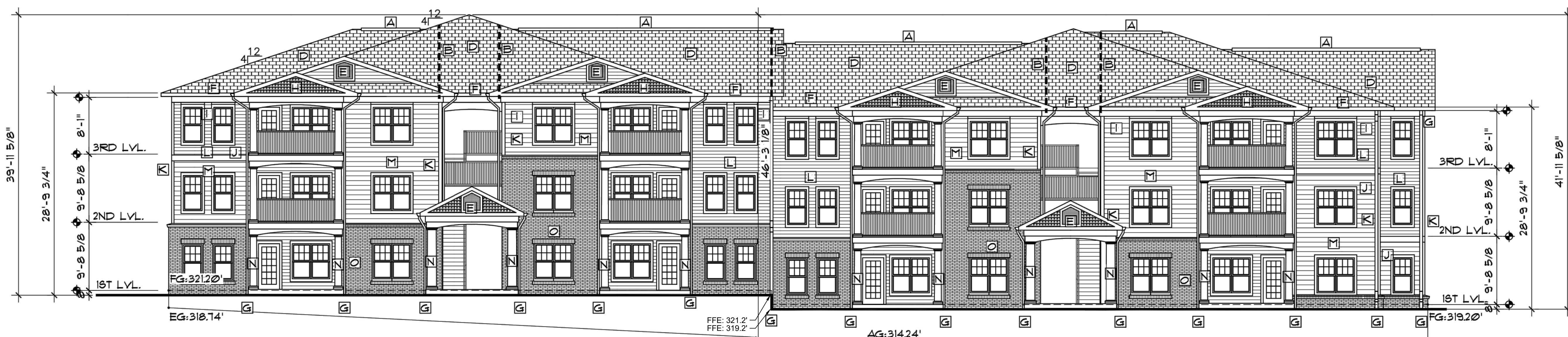
1 BUILDING #200 PARKING ELEVATION (WEST) 1/8" = 1'-0"
