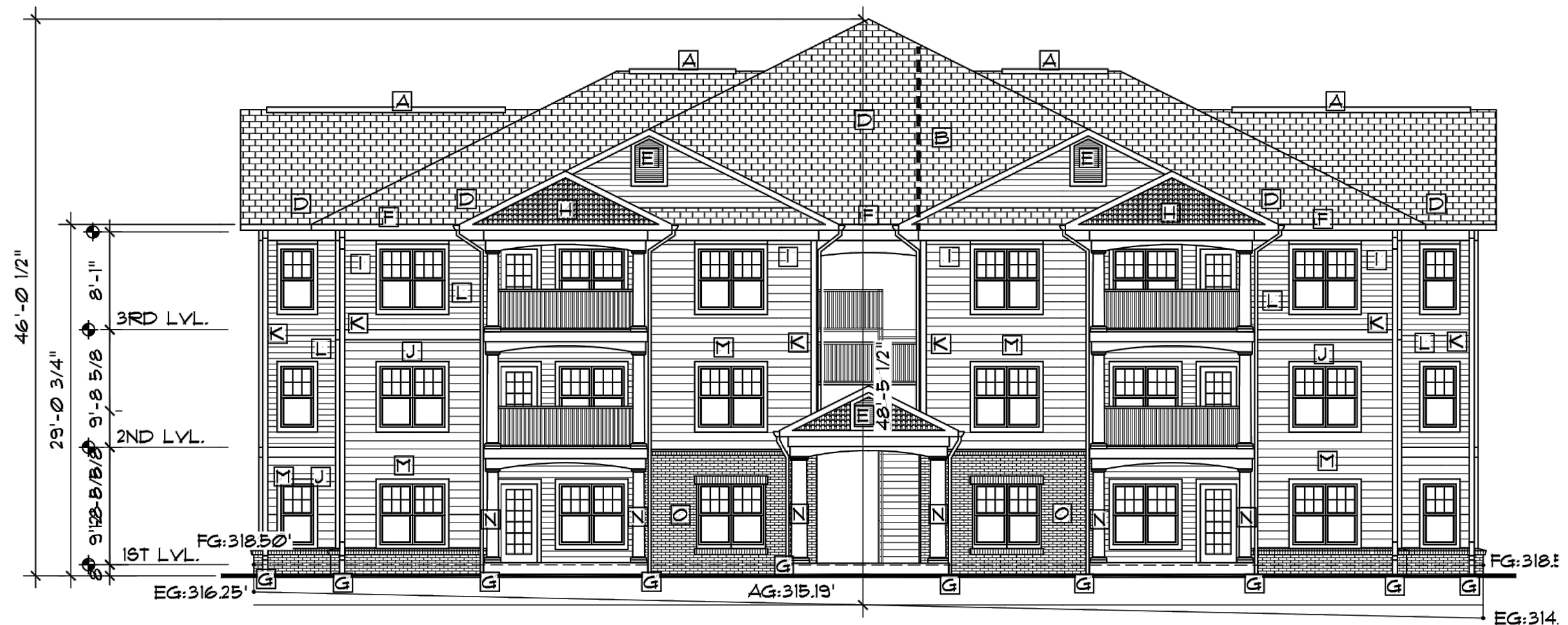
2 BUILDING #500 FRONT AND REAR ELEVATION (WEST) 1/8" = 1'-0"
