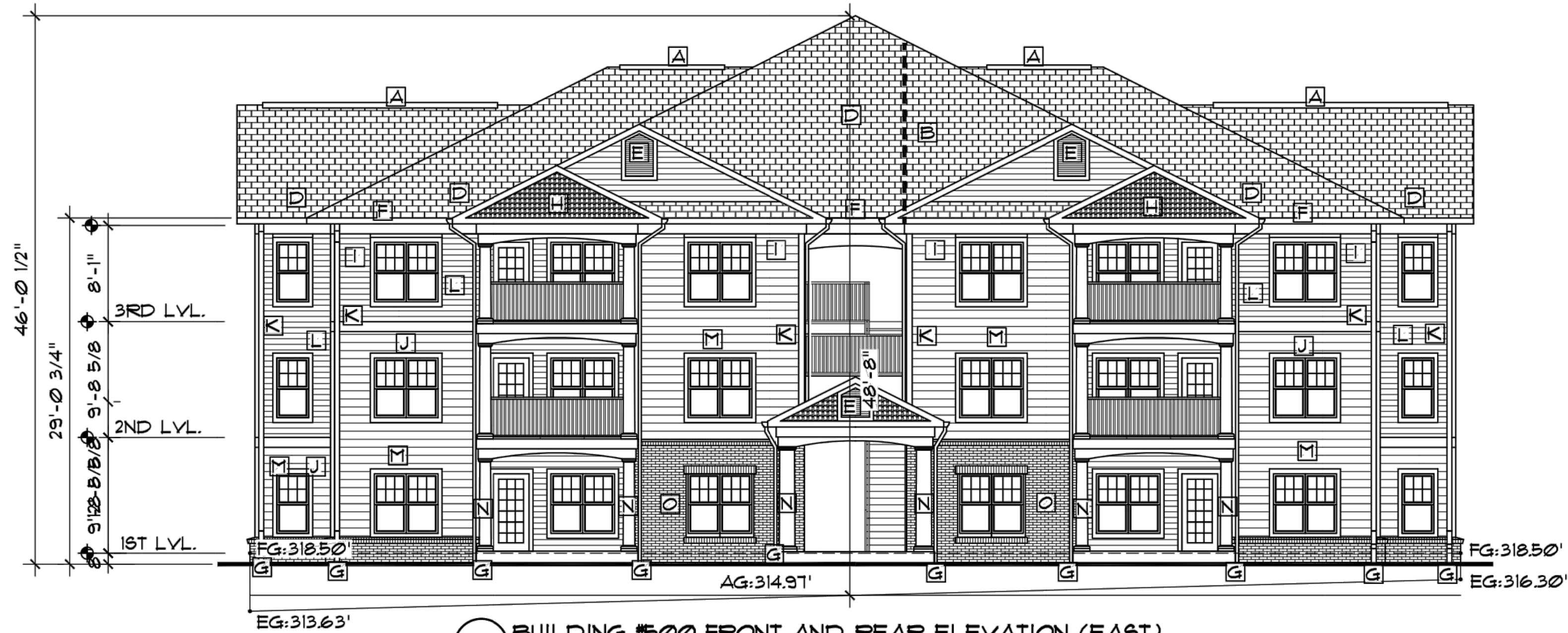
4 BUILDING #500 FRONT AND REAR ELEVATION (EAST) 1/8" = 1'-0"
