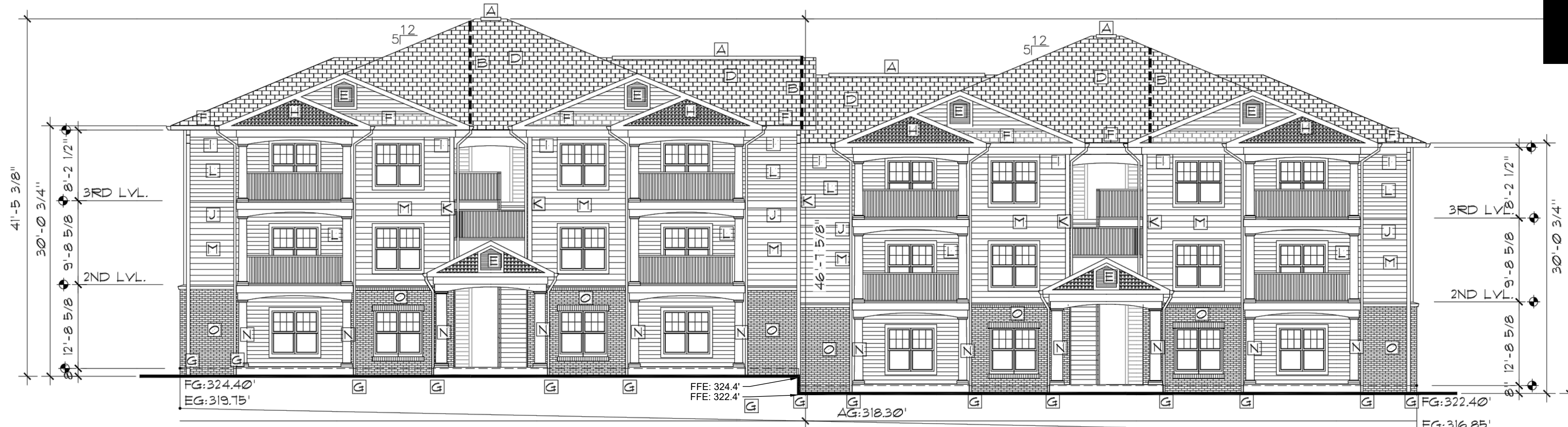
4 BUILDING #400 STREET ELEVATION (WEST) 1/8" = 1'-0"
