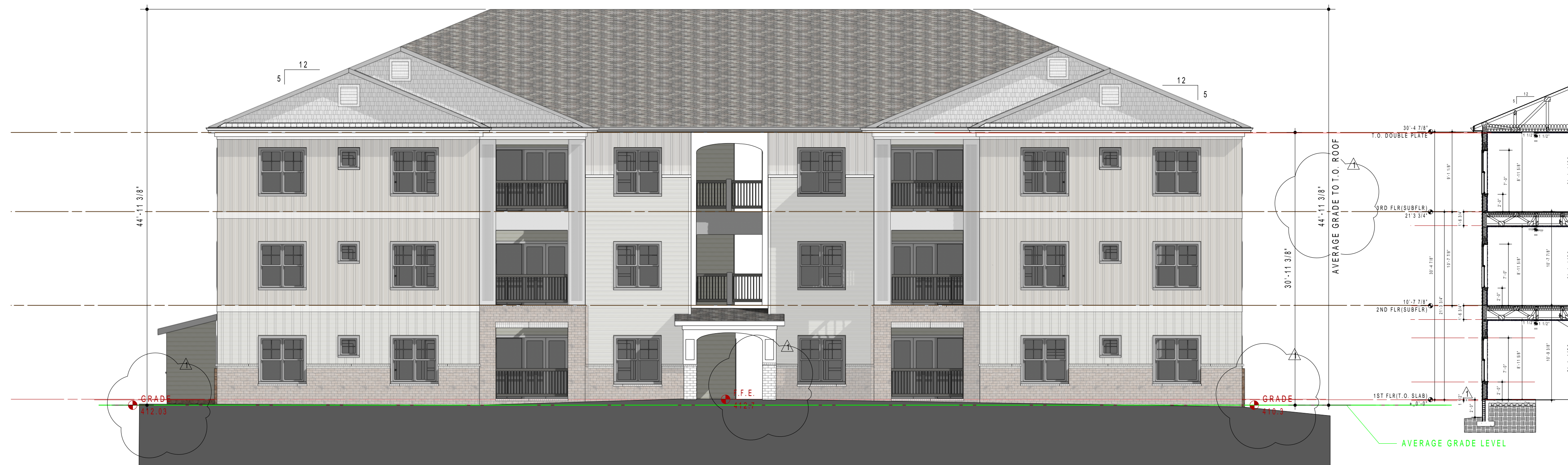
1 BUILDING 2-TRYON ROAD (SOUTH) ELEVATION Scale: 1/8" = 1'-0"
