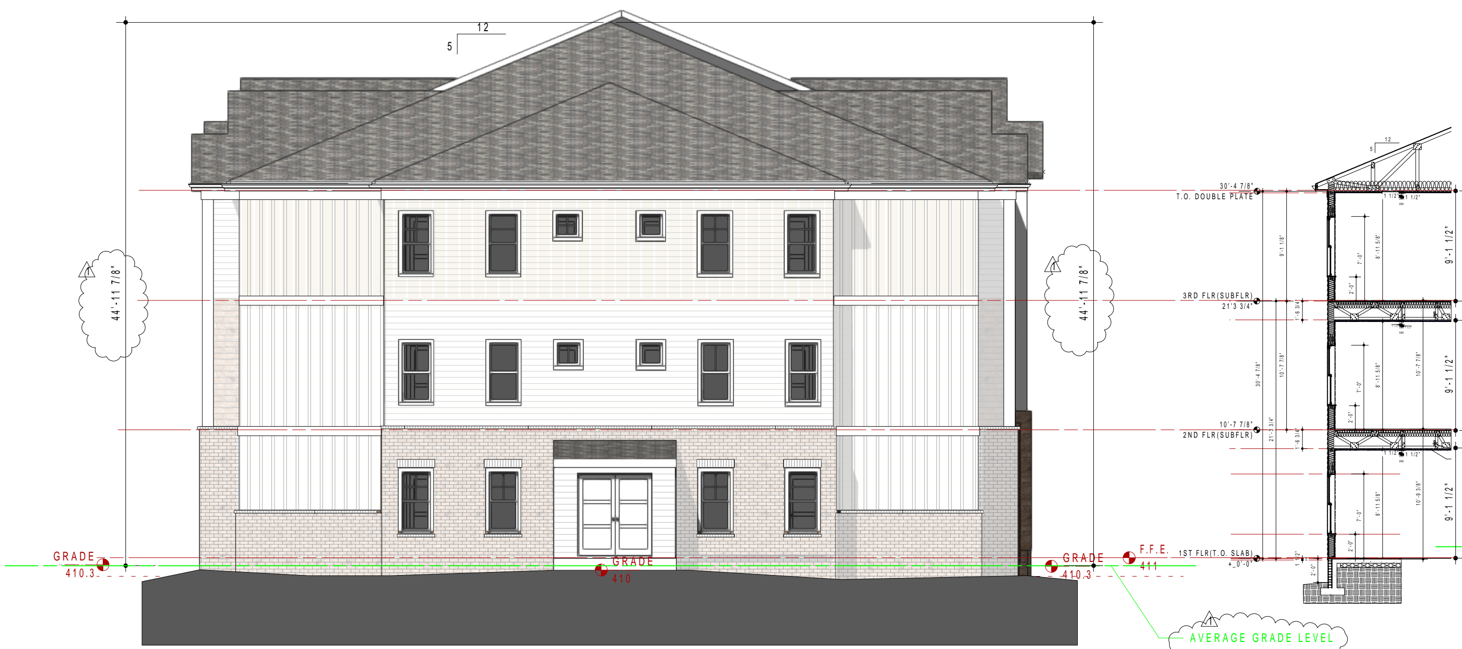
4 BUILDING 1-SOUTH-EAST ELEVATION Scale: 1/8" = 1'-0"
