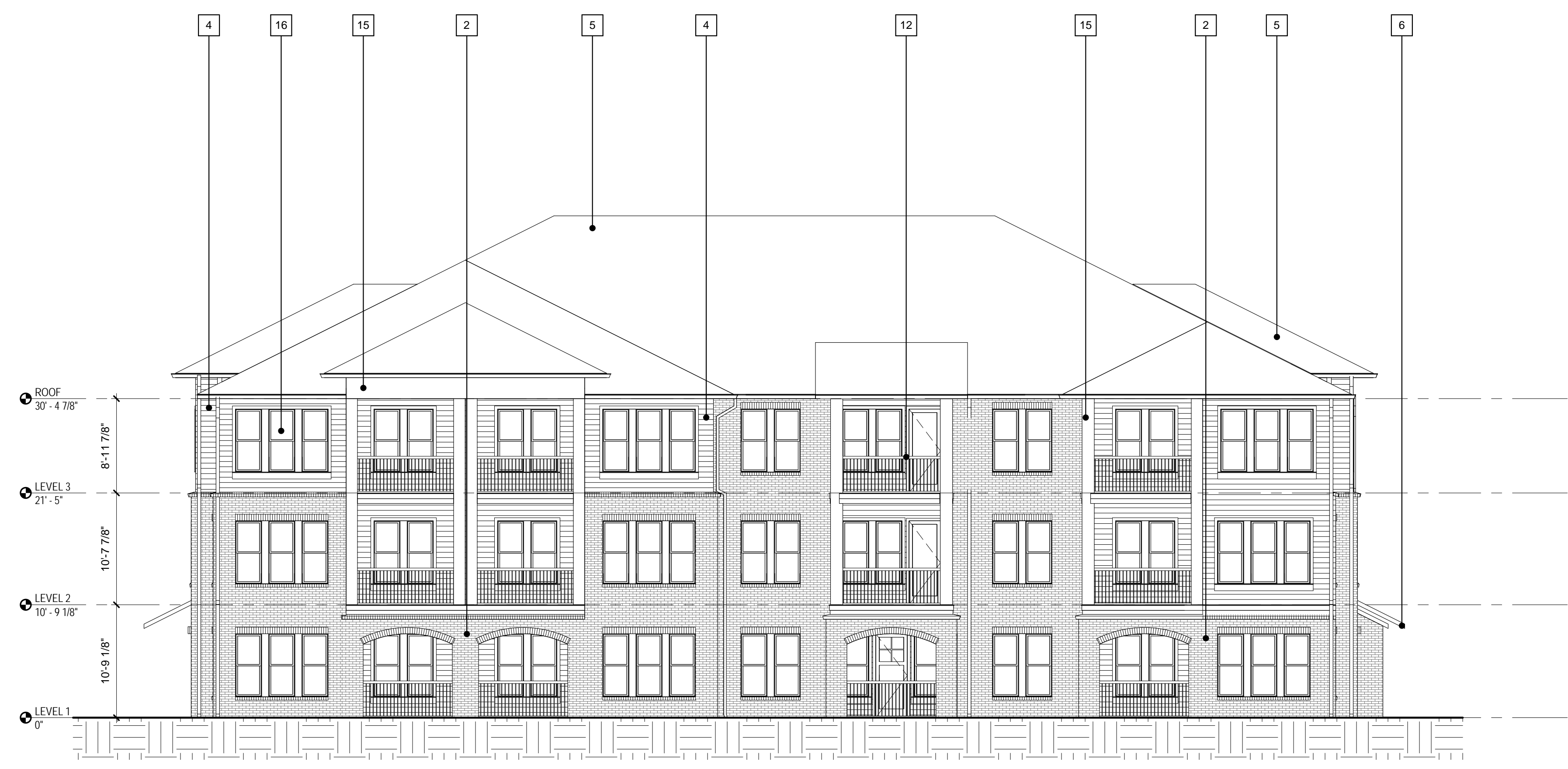
1 BUILDING 5 - WADE PARK BOULEVARD ELEVATION - CE SCALE: 1/8" = 1'-0"
