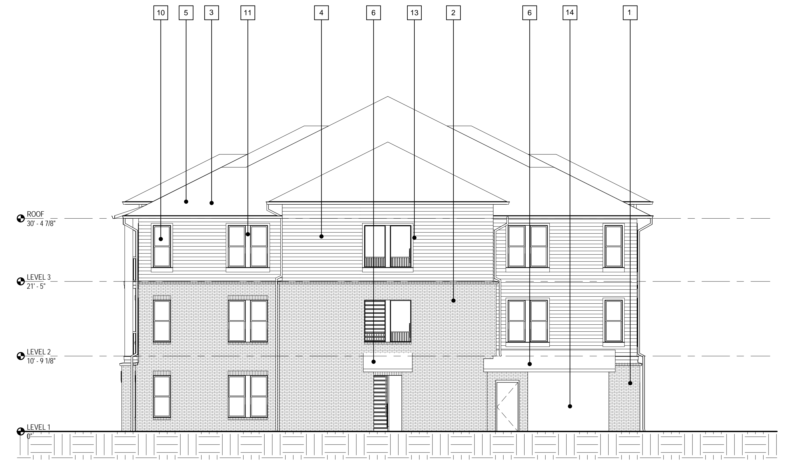
3 BUILDING 5 - NORTH ELEVATION - CE SCALE: 1/8" = 1'-0"
