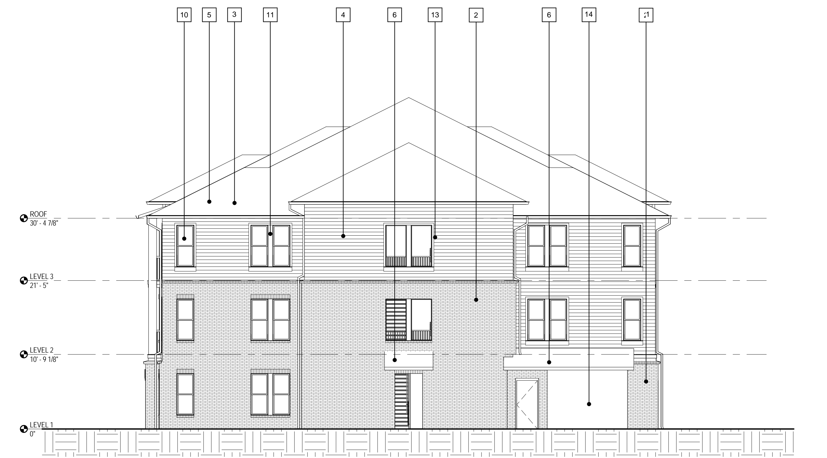
4 BUILDING 2 - NORTH ELEVATION - CE SCALE: 1/8" = 1'-0"
