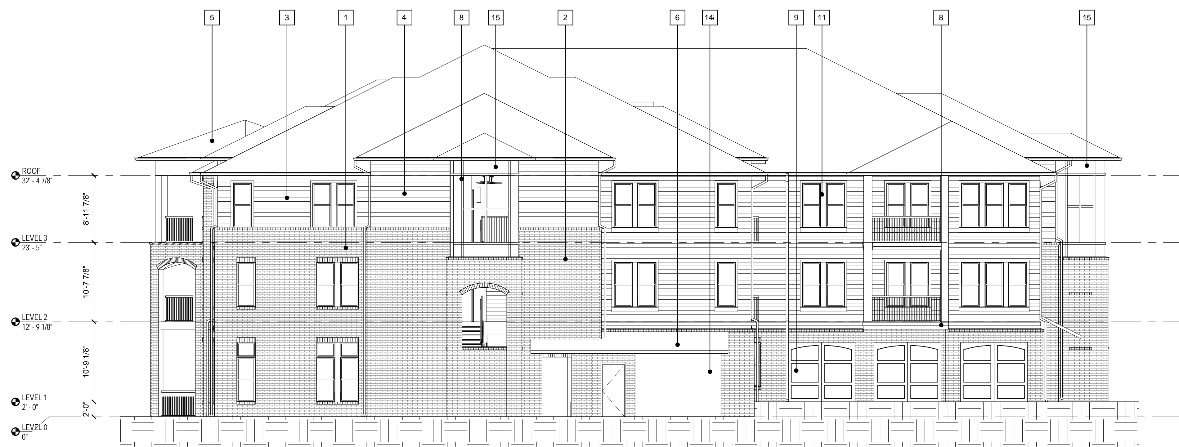
2 BUILDING 3 - SURFACE PARKING ELEVATION - CE SCALE: 1/8" = 1'-0"
