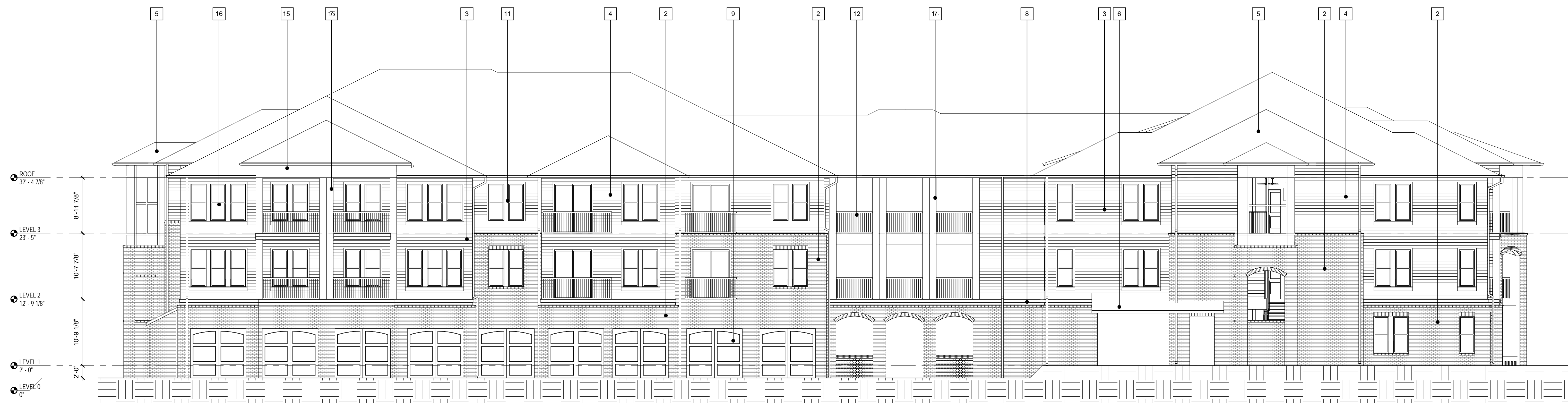
2 BUILDING 3 - GARAGE PARKING ELEVATION - CE SCALE: 1/8" = 1'-0"
