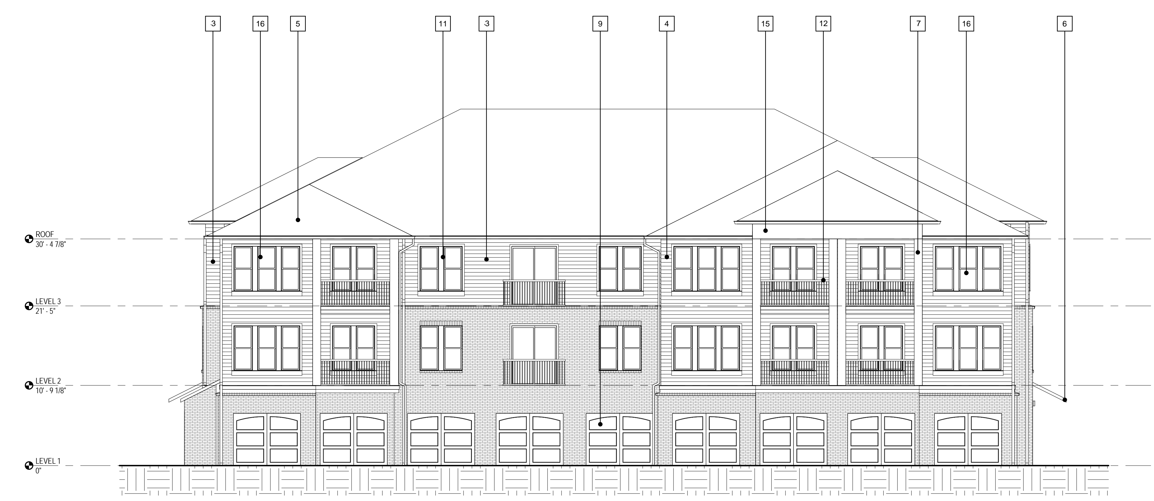
4 BUILDING 1 - SURFACE PARKING ELEVATION - CE AE3.10 SCALE: 1/8" = 1'-0"
