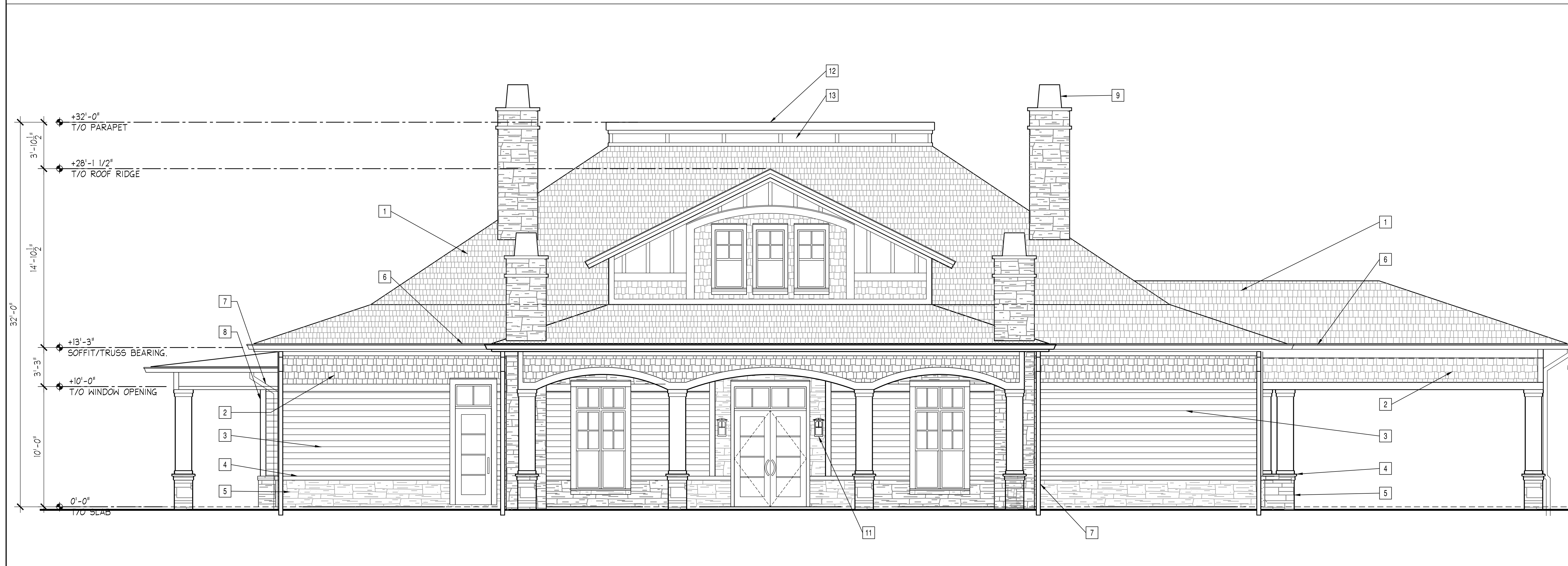
1 CLUBHOUSE - POOL ENTRY ELEVATION (WEST) Scale: 1/4" = 1'-0"
