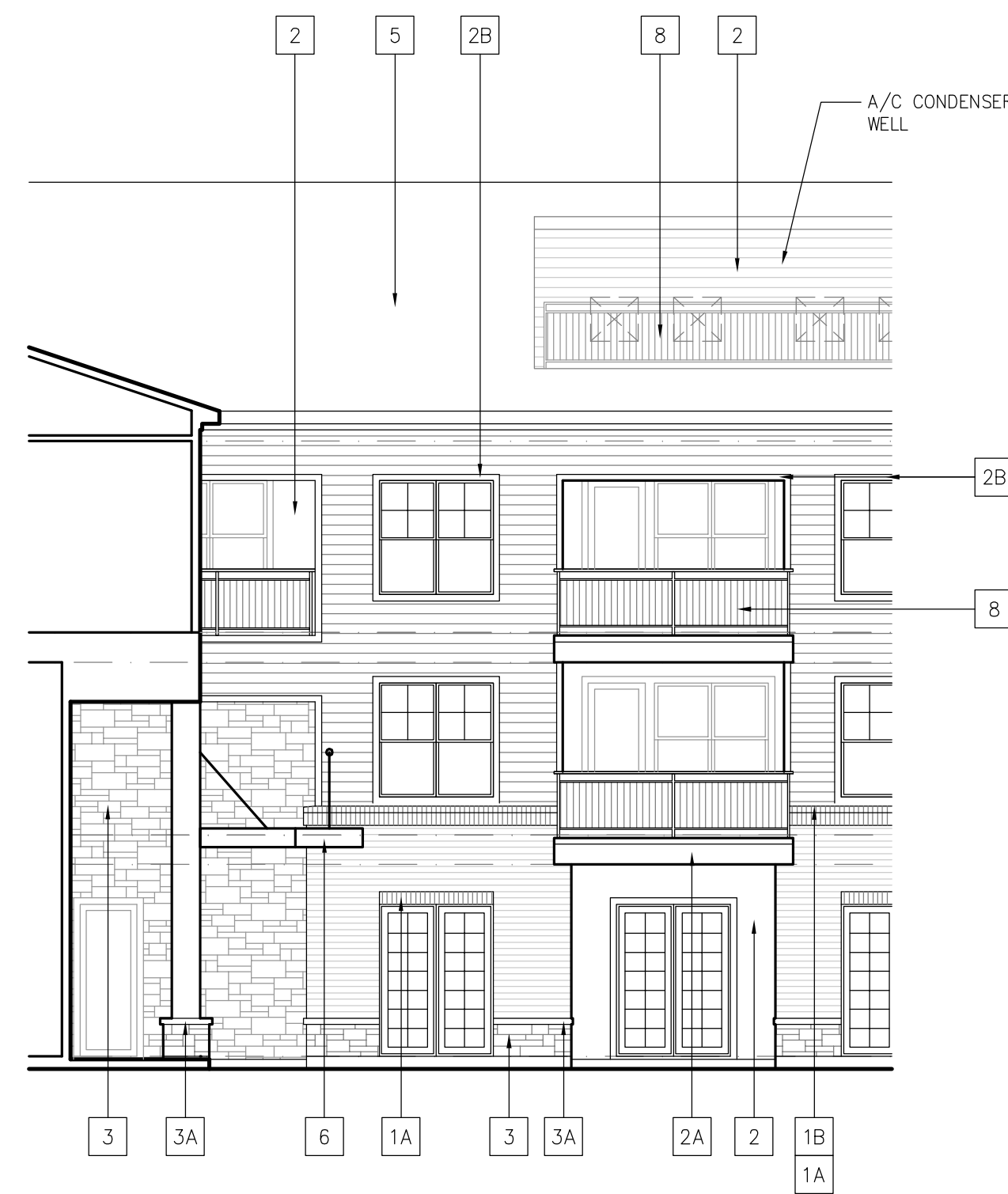
3 PARTIAL NORTH COURTYARD ELEVATION 1/8"=1'-0"
