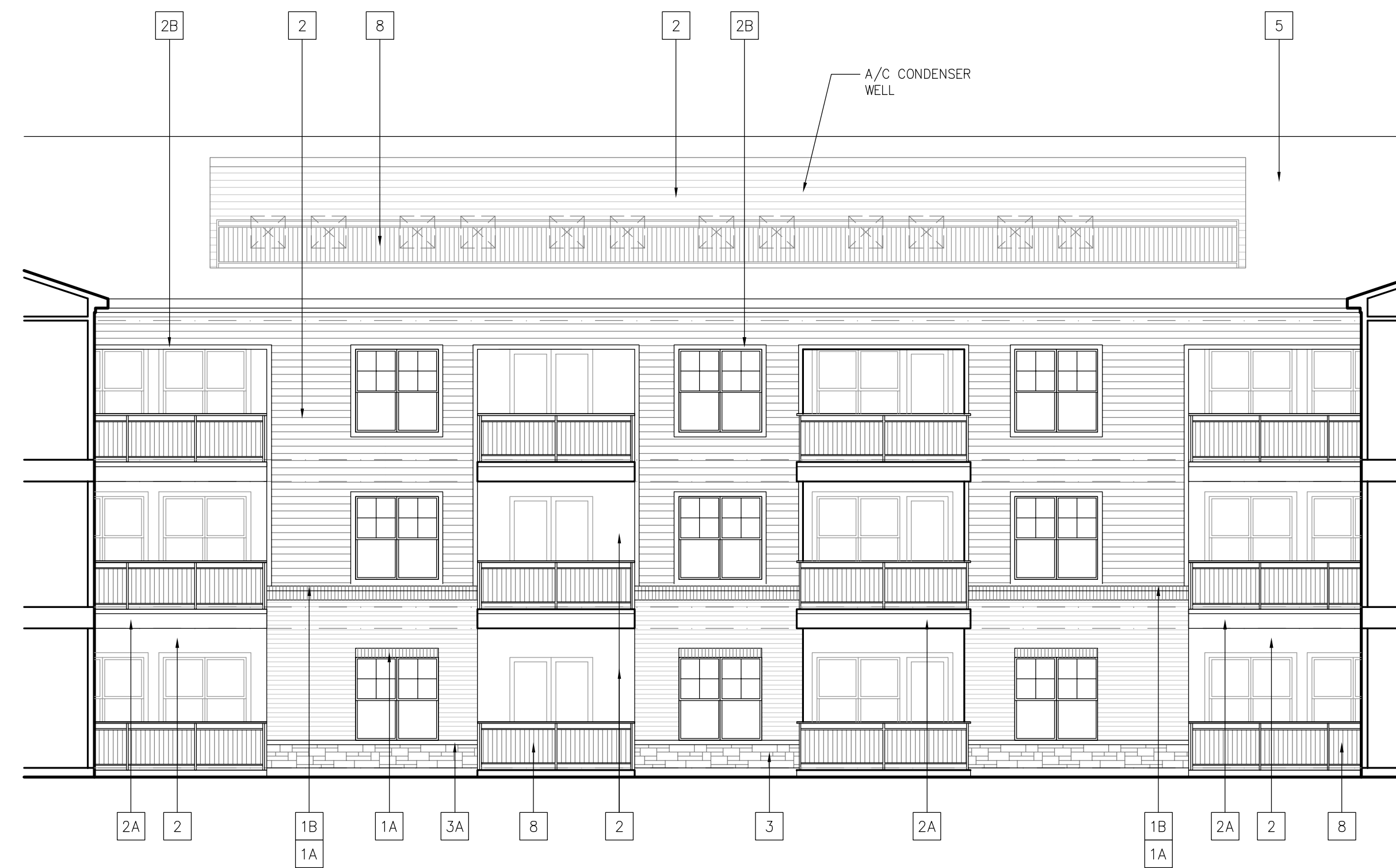
2 PARTIAL EAST COURTYARD ELEVATION 1/8"=1'-0"
