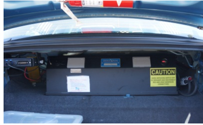
Anti-Idling Device in trunk of police cruiser
